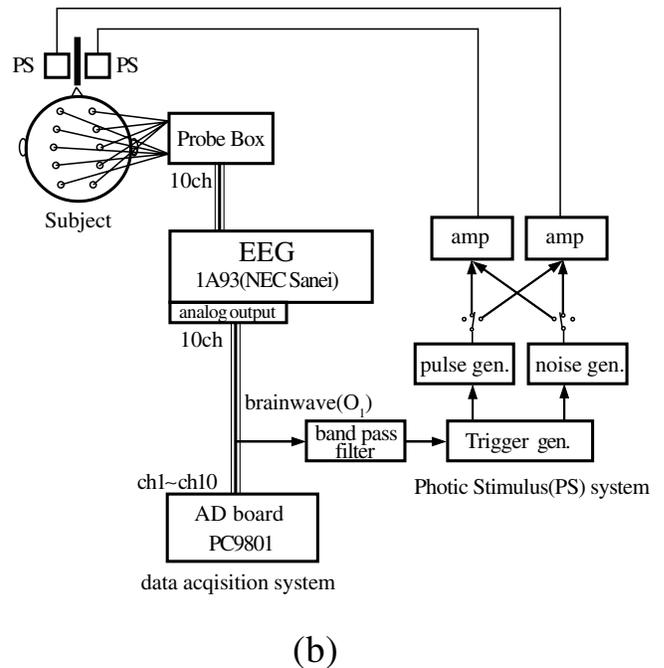
FIG. 2. International 10–20 electrodes arrangement (a) and experimental setup (b) for measurement of brain waves. Following the 10–20 international electrode system, target electrodes in this study were positioned at ten fixed points on the scalp using the linked-earlobe references.
